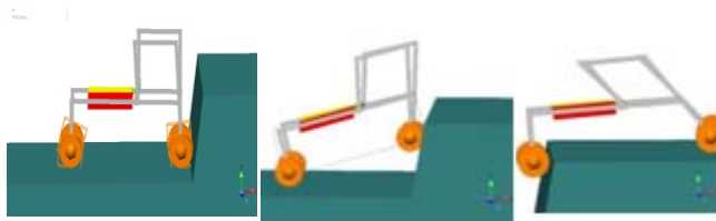
Figure.4a(left).Rigid suspension unable to negotiate a step like discontinuity. Figures 4b, 4c. A torsion based suspension mechanism able to negotiate discontinuity
