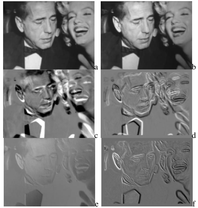
Fig. 10. Influence of luminance variation (a) desired image (b) final image \mathbf{r}^* (c) initial error in the intensity space (\mathbf{I}(\mathbf{r}) - \mathbf{I}(\mathbf{s}(\mathbf{r}))) and (e) initial error on the norm of the gradient used in the control law (\|\nabla \mathbf{I}(\mathbf{r})\|^2 - \|\nabla \mathbf{I}(\mathbf{r}^*)\|^2) (e) final error in the intensity space and (f) final error on the norm of the gradient used in the control law.
