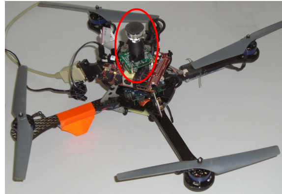
Fig. 1. Omnidirectional camera (highlighted by the red ellipse) on a flying robot. The USB camera is connected to a “Beagle Board” computer (see http://beagleboard.org ) that controls the four-rotor flyer.
