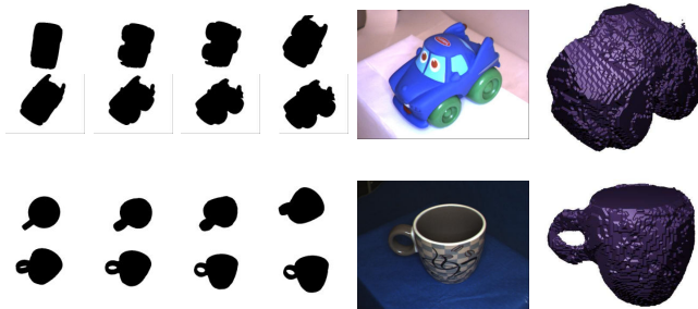
Fig. 8. 8 of the 10 silhouettes, one camera view and a rendering of the reconstructed model for real objects.
