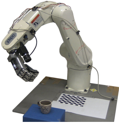
Fig. 1. Six degree-of-freedom manipulator with an eye-in-hand camera
