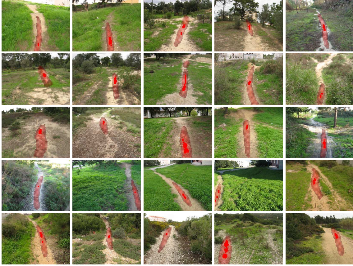
Fig. 4. Data-set representative frames. Each image corresponds to one video whose ID is given by increasing order from left to right and top to bottom. The overlaid red blobs represent the model’s estimate of the trail location, which corresponds to an activity of the neural field above 0.85.
