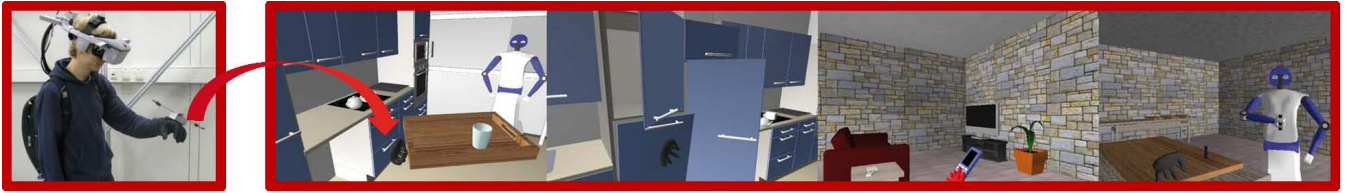
Fig. 3. Left: Human with head and hand tracking devices and data glove. Right: example impressions of the 1st person view of the virtual environment.
