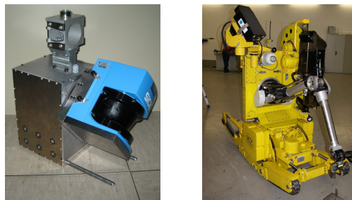
Fig. 2. (left) RoSi: Rotating SICK laser scanner system, (right) LMF: radiation-tolerant teleoperated service robot.
