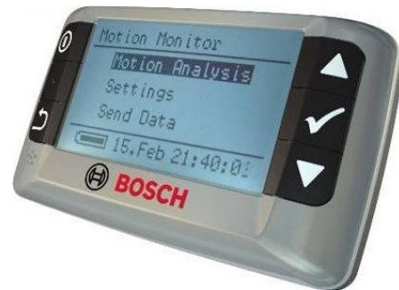
Fig. 1. The mobile footstep sensor carried by the user. Dimensions are 8.5 x 5 x 2 cm (width x height x depth).
