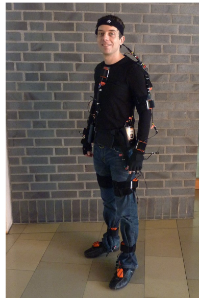
Fig. 2. A person wearing the motion capture suite which provided ground truth data to analyze the mobile footstep sensor. We also used this suite to record the leg movements of people used in the experiments.
