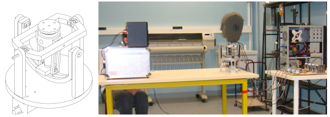
Fig. 4. System overview: (Left) The 3 DOF mechanical system reproducing the three rotations of a human head; (Right) Experimental setup, from the loudspeaker on the left to the acquisition card on the right.
