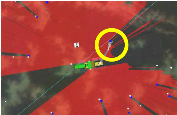
Figure 6: The Virtual Testbed brings up the problem that the harvester's felling aggregate will be disturbing the scanning process.
