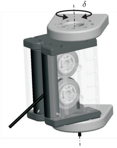
Fig. 2. Deflection unit for a tendon-based robot
