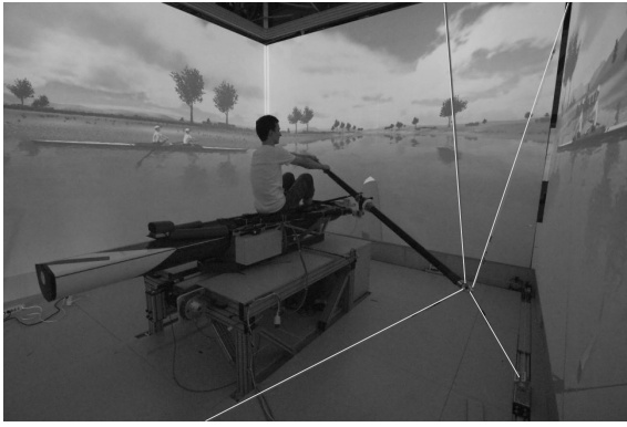
Fig. 4. Rowing simulator with the r^3 -system as a haptic interface
