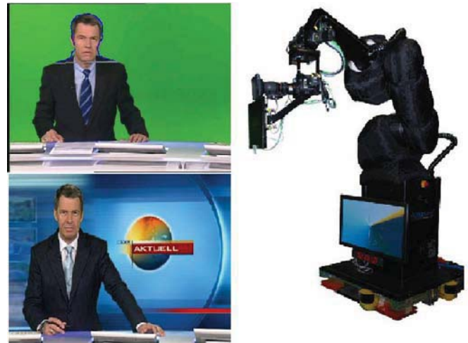
Fig. 1. A virtual set for daily news broadcasting events. The upper and lower left pictures show the virtual studio. The right shows our robot camera system for broadcast automation. (image courtesy: RTL Television Studio Köln, Germany, and Robotics Technology Leaders GmbH).
