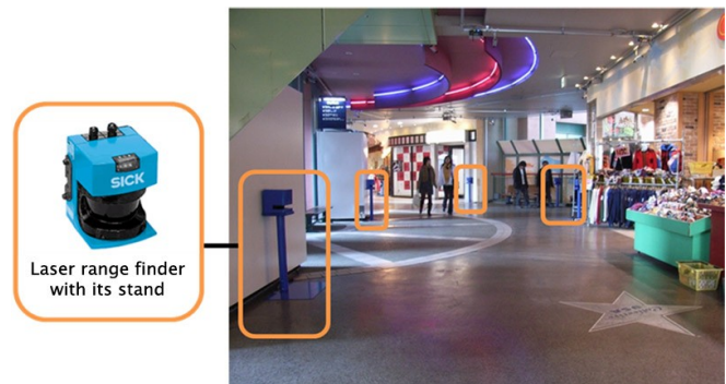
Fig. 3. Mounting stands for laser range finders in the field environment.
