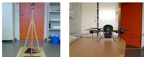
Fig. 1. Experimental setups: A ground vehicle with a USB camera and an AR-100 UAV with onboard camera.
