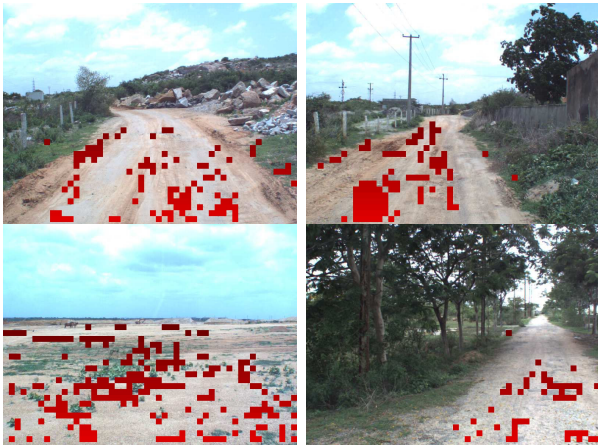
Fig. 6: Test images marked with red-colored-patches, representing the labels that are correctly labelled by Adaptive algorithm but wrongly labelled by offline Partition method.
