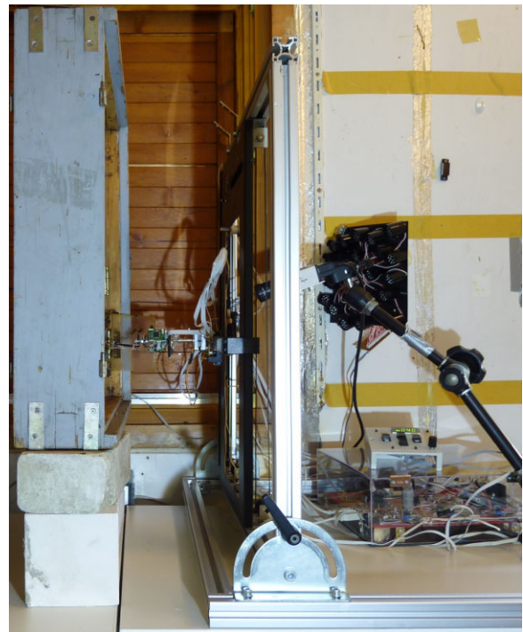
Fig. 2. Experimental setup. The observation hive has four windows we can open to insert the bee sized body of the robot. The body can be moved with an x/y positioner that is mounted vertically in an aluminium frame.
