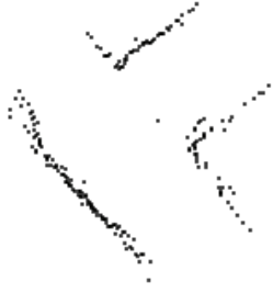
Fig. 4. Example of local map built by letting the robot rotate over 360^\circ .
