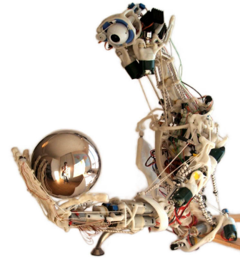
Fig. 1. ECCE, a so called anthropomorphic robot, is the platform for the work presented here. In this type of robot not only the outside of the human body is copied but also the inner structures, like bones, joints, muscles, and tendons.
