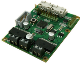
Fig. 5. The electronic control unit (ECU) running the distributed controllers, which was specifically developed for this project.
