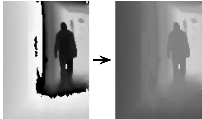
Fig. 1. Unwrapping the input depth image (left). The brightness encodes the measured distance (dark pixels are near, bright pixels far away). The abrupt change from bright to dark in the input image is the phase jump that we want to detect in order to correct the measured distances and to obtain the unwrapped depth image (right).
