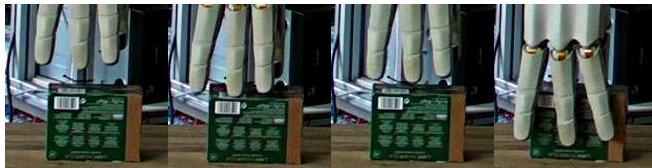
(a) Approach, collision, pull-back, grasping using the corrected pose.
