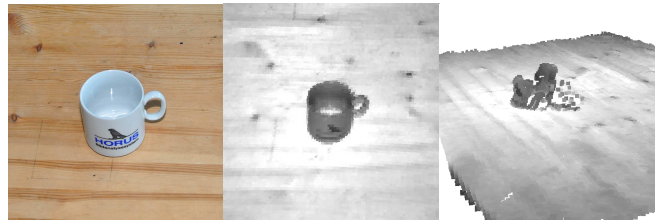
Fig. 4. The robot observes a cup. On the left, an RGB camera image, and on the right, two different views from the point cloud data.
