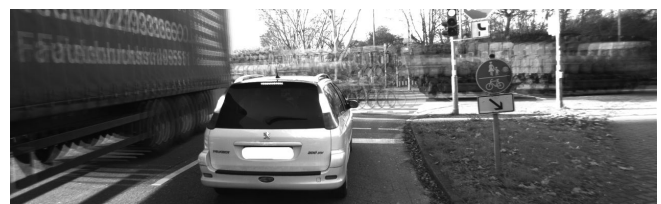
Fig. 1: Moving objects make egomotion estimation difficult.
