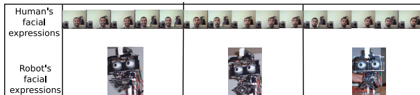
Fig. 5. The robot is able to recognize the facial expressions when the human's partner is at a distance of 2 m.
