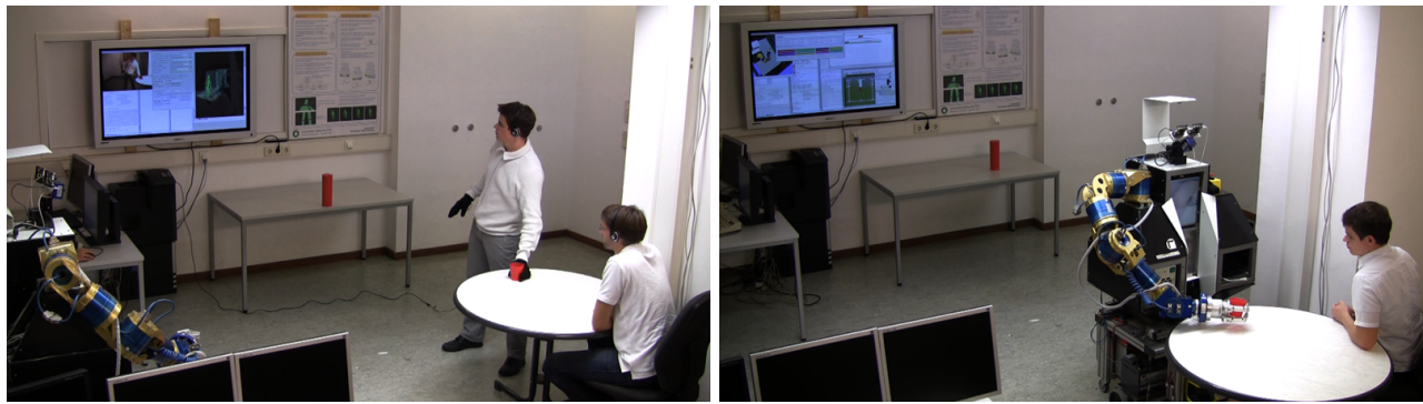
Fig. 4. Demonstration of Mission 1 by robot actor and human actor with actively watching robot (left) and autonomous execution with the robot and interacting human (right). Gloves improve in-hand object localization and headsets improve speech recognition during the demonstration phase. See accompanying video for an example of demonstration and execution of Mi1 and Mi2.
