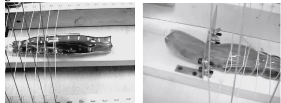
Fig. 3. Everting toroid using contracting rings actuators for propulsion, and for traversing a hole.
