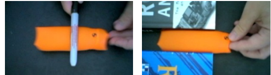
Fig. 2. Fluid filled toroid model demonstrating the ability to squeeze under obstacles and through holes.
