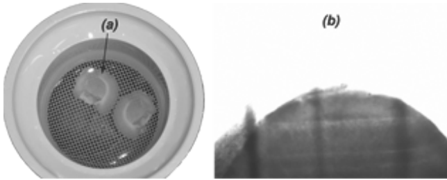
Fig. 9. (a) Prepared slice before being used, (b) Slice under the 4\times dry objective; (the actual width of the image is 2.151mm ).
