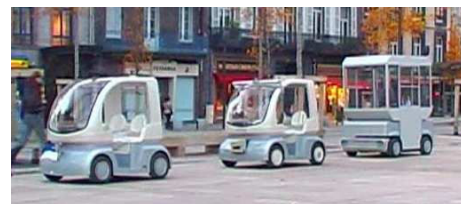
Fig. 1. Experimental vehicles: two Cycab leading a RobuCab
