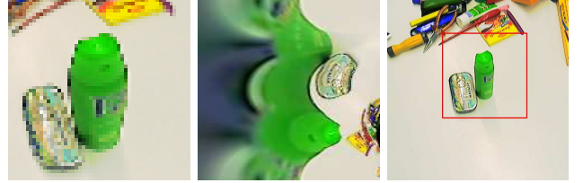
Fig. 3. Emulated foveal vision. The left image shows the transformed input image. As one can clearly see the resolution at the center is higher. In the middle the representation in log-polar coordinates is displayed and on the right the input image is shown, the red square shows the region of interest that is transformed. The size of these images are 52 \times 52 for the foveal image, 164 \times 164 for the log-polar image and 219 \times 219 for the region of interest.
