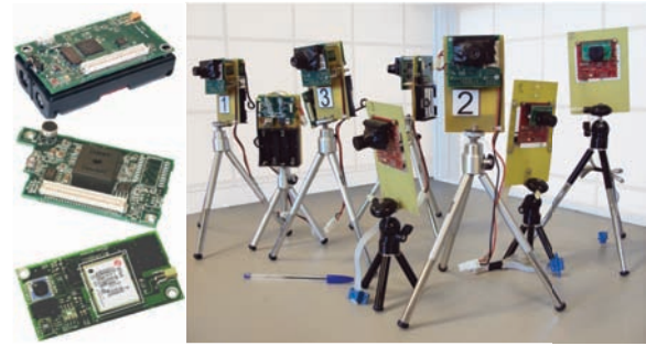
Fig. 3. Left) Xbow Mica2 node with MTS400 and MTS300 sensor boards. Right) Set of five CMUCAM3 and three CMUCAM2 .
