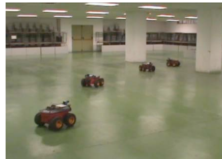
Fig. 11. Network repair experiment in the testbed indoor scenario.
