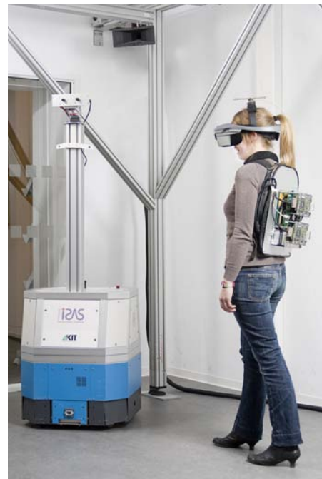
Fig. 1. Telepresence environment at the ISAS Lab: Teleoperator Omnibase and user wearing the tracking system. Sound signals travel from four speakers (mounted in the corners of the room) to four microphones (mounted on top of the HMD).
