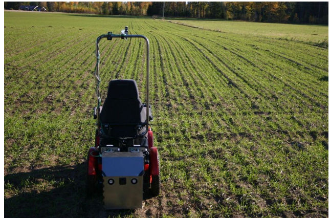
Fig. 1: Mobile experimental robot on a row-structured agricultural field
