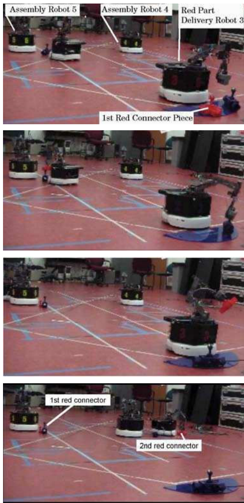
Fig. 13. Snapshots of a test run of the even demanding mass delivery scenario. Assembly robots begin positioned at 2 different points of highest demand for parts. As the red connector parts are delivered, the maximum demanding mass for the entire map changes, causing the delivery robot to change delivery targets, first to robot 5, then to robot 4.
