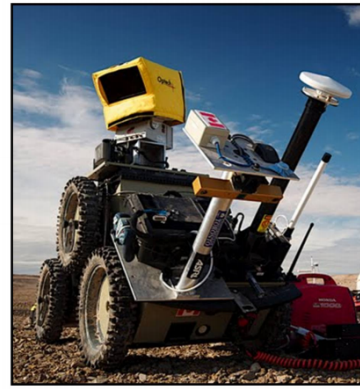
Fig. 5: A sample SOP plan at a planetary analogue site is shown on the left. A long-range point cloud was collected using an Optech ILRIS, shown mounted on the test robot at the right. Plane-fit terrain assessment was used for the low-fidelity assessment. The gray, yellow and red planes respectively show traversable, uncertain and obstacle regions of the terrain. The naïve (dashed) and SOP (solid) plans are shown. The initial reassessments requested by SOP yielded obstacles so an alternate path was proposed, assessed, and found to be traversable. Times are the total of all cost contributions.
