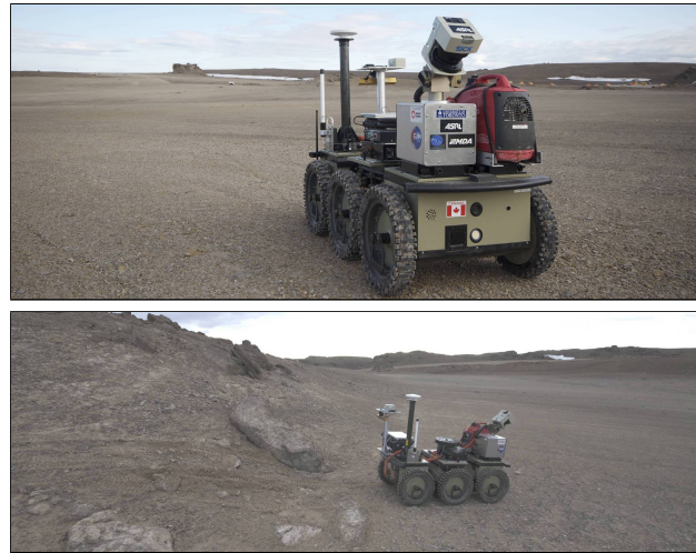
Fig. 1: Mobile robots can operate in terrain of varying difficulty. Some areas are easily assessed (as in the top image), while others require more advanced methods before the traversability can be determined (bottom image).
