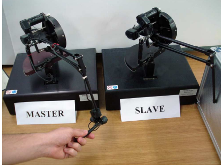
Fig. 4: Experimental Setup with a pair of Phantoms 1.5.
