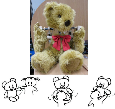
Fig. 3. The picture of our teddy bear social robot which is built based on the hybrid passive-active compliant motion system and aims at playing with children physically with a sense of interactivity and naturalness. The figures below demonstrated how the robot could cope with children's unpredictable behavior with the effect of hybrid compliant motion system.
