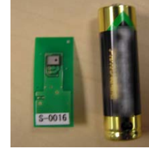
Fig. 5. A MEMS microphone module with an AAA battery. The center part of the module is microphone unit (Knowles SPM0406HE3H).
