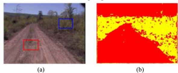
Fig.1.Result of Window-based Learning Algorithm. (a).Sampling windows image. Red window contains positive training set while blue window contains negative training set. (b). Result of Classification. Red pixels are positive class while yellow pixels are negative class.
