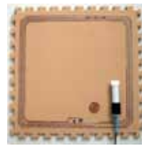
Fig. 2. Reader antenna and a tile of a cork mat with a tag
