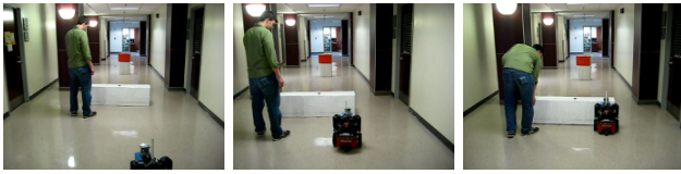
Fig. 7. Left: The human gets ready to push the box on the left side. Center: The robot moves into position to help push on the right side of the box. Right: The human and the robot work together to push the box.
