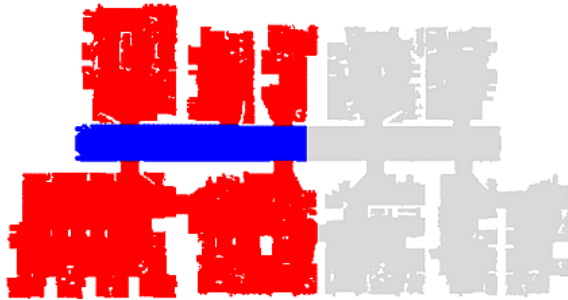
Fig. 1. Training dataset: the grey points depict the background map as a reference. Red and blue points are observer's positions which are manually labeled as in room and corridor respectively.
