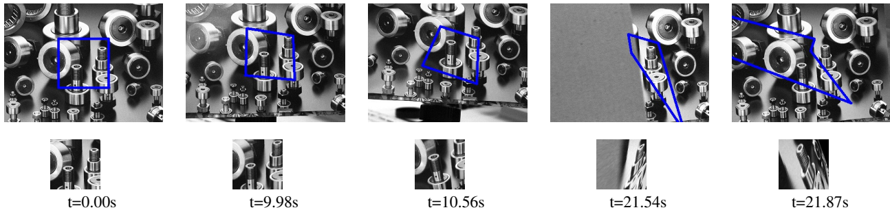
Fig. 7. CPU-ESM tracking. The change of warped images shows that CPU-ESM tracking can not track the same moving object as in Fig. 6 when the object moves fast or occlusion happens.
