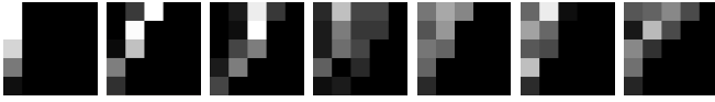
Fig. 6: Radius-based Surface Descriptors (RSD): 2D histograms of normal angle difference and distance from a reference point to its neighbors (examples are shown from left to right for histograms computed for points on a plane, sphere, corner, edge and three cylinders, where the last two are computed for different points of the corrected teapot scan presented in Figure 4) – from these histograms the physical surface radiuses can be read as the slopes of the different lines going through the lower left corners.
