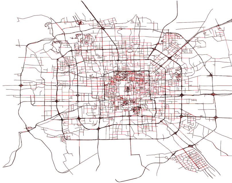
Fig. 1: The main idea in this paper is to combine the advantages of direct and iterative methods: we identify a subgraph that can easily be solved using direct methods, and use that as a preconditioner in conjugate gradients. This is illustrated above with a map of Beijing, where the subgraph is a spanning tree (in black), and the remaining loop-closing constraints are shown in red.
