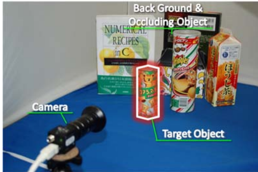
Fig. 8. Experimental Setup of Target Object Detection with Occlusion
