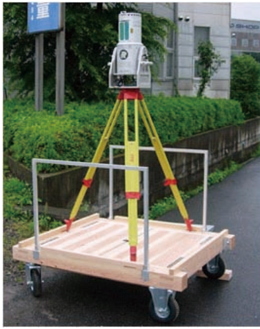
Fig. 1. LMS-Z420i Scanner Mounted on a Cart
