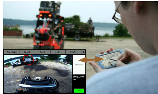
Fig. 3. Forklift being commanded, via the tablet interface, to pick up a pallet from a truck bed.
