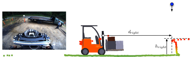
Fig. 7. Truck bed detection algorithm depicted on the raw data acquired from sensor mounted to the right of the mast.
