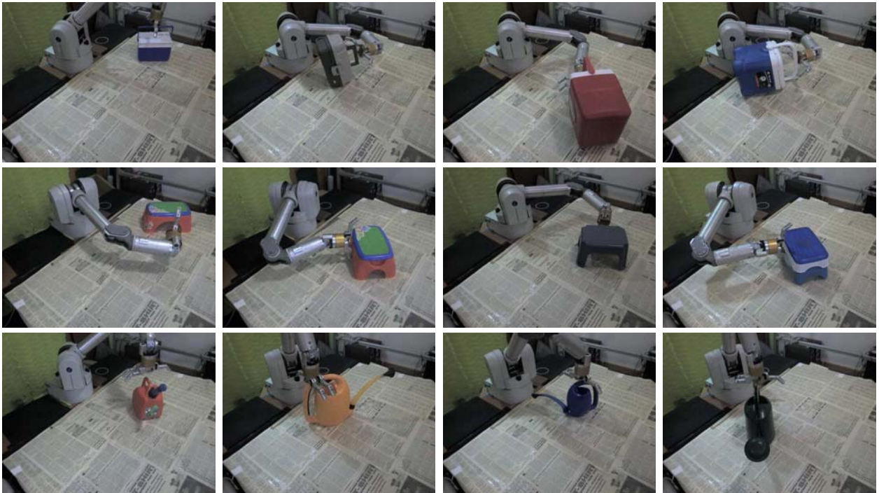
Fig. 10. Four grasps for each of the three classes (from top to bottom: coolers, stools, and watering cans).
