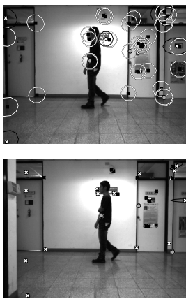
Fig. 6. The experimental results. (a)(b)(c) showed the stereo image pairs and the results at frame 136, 315 and 468. The upper image is the right camera view and the lower image is the left camera view. In the image, Black solid squares and grey circles indicate map features and moving objects with associated new measurement and being updated. The white ellipses show the projected 2\sigma bounds of the estimates of the map features and moving objects. White cross with its black uncertainty bound indicate map features without any associated measurement and not being update. The result showed three moving persons were tracked with a small depth uncertainty.
