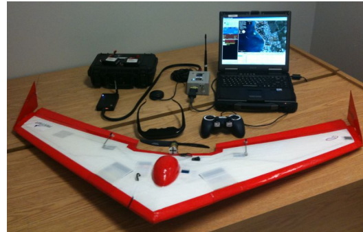
Fig. 1. The Procerus ® Unicorn is a fixed-wing unmanned aerial vehicle with an on-board autopilot microprocessor and gimbal-mounted camera.
