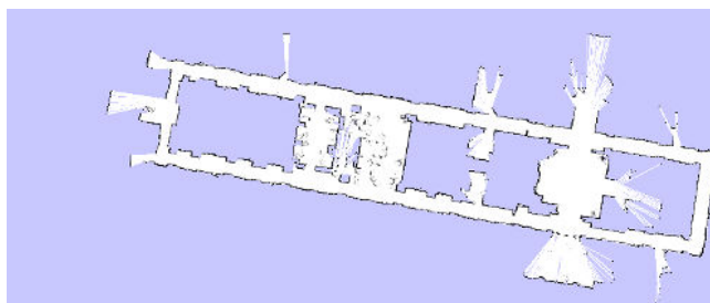
Fig. 2. 2-d map of the environment used in these experiments, as produced by GMapping and the robot shown in Figure 1
