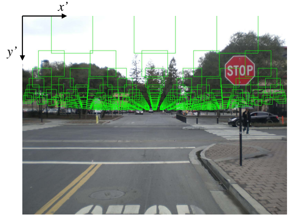
Fig. 3. Projection of various possible 3D traffic sign locations into the 2D image plane using (2).
